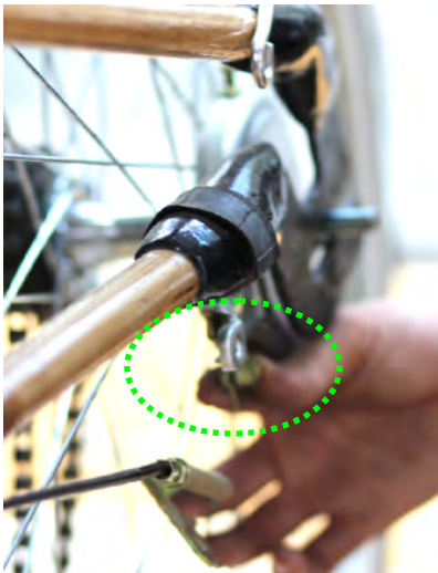
Attach brake clip to secure brake line
