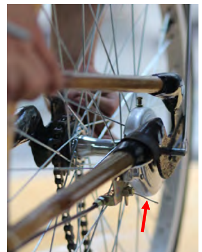
Tighten brake cable by pulling brake cable tightly through brake housing
