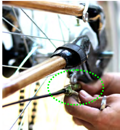
Pass rear brake cable through rear wheel eyelet
